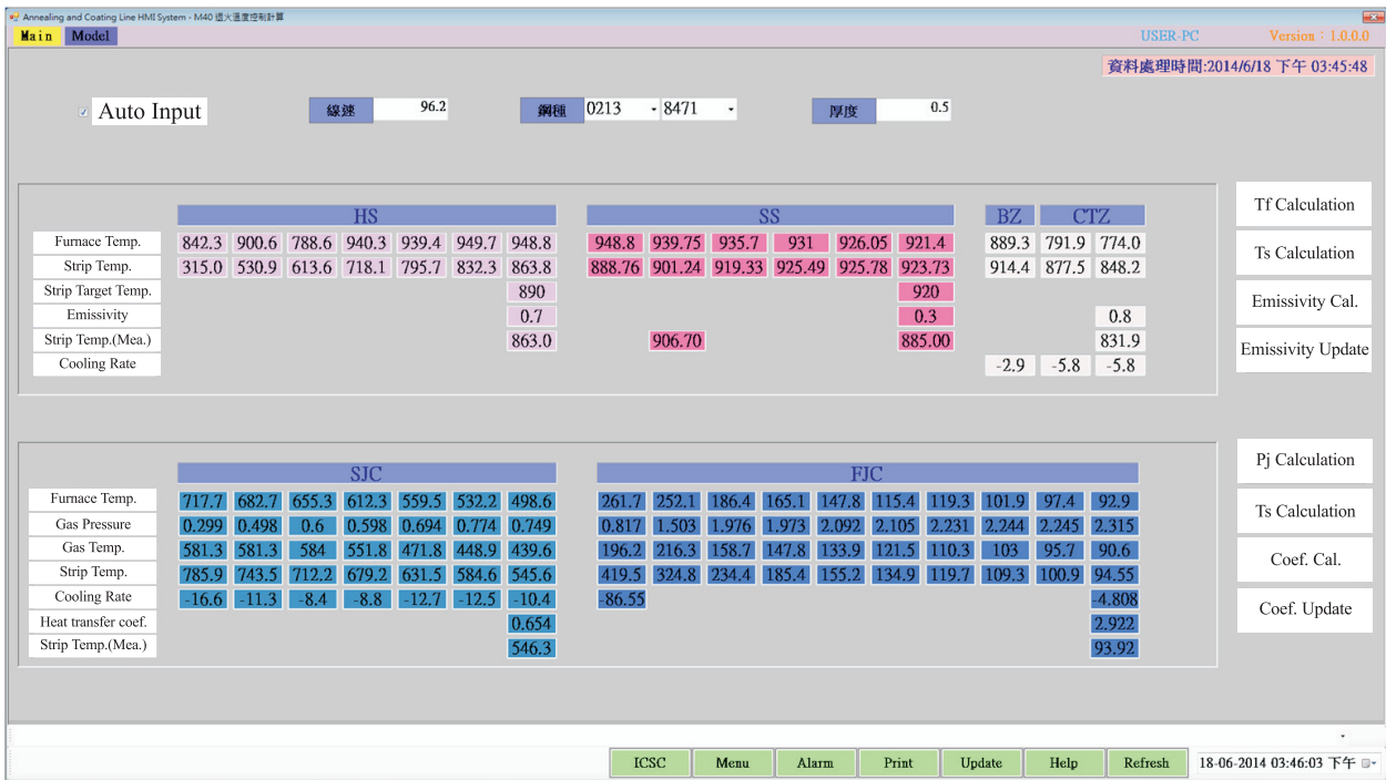
Fig.8. The pilot calculation for strip temperatures, furnace temperatures, gas pressures and emissivity.
